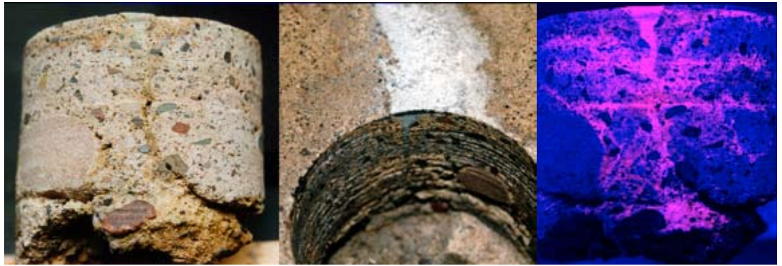
Concrete core sample taken from concrete repaired with Roadware 10 Minute Concrete Mender. Examination under filtered UV light shows deep penetration and full depth repair.
