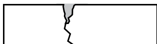
Finished repair is open for all traffic. Any staining due to over banding will quickly wear off or can be removed with a light sanding.
