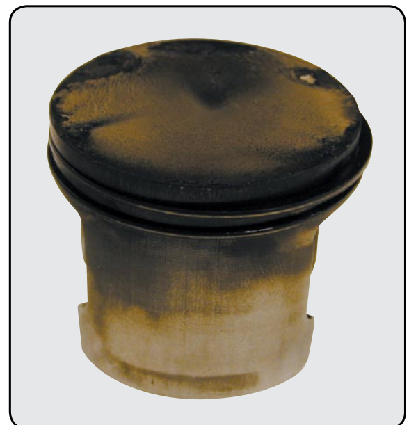
Piston Tested with Leading Brand 2-Stroke Oil
