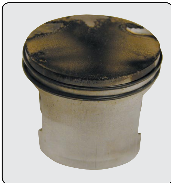
Piston Tested with ICS 2-Stroke Oil
